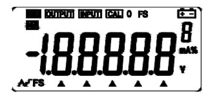
OUTPUT : Press the key OUTPUT / IN / SW when the symbol OUTPUT appears. It denotes that the Instrument is in a state of output.
